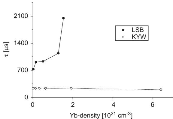
Fig. 3. Fluorescence lifetime of Yb:KYW and Yb:LSB versus Yb concentration; for LSB the Yb concentrations are given only for the La sites.
