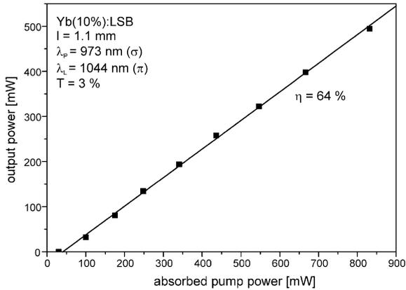
Fig. 6. Input–output curve of Yb:LSB in a linear resonator under TiSa pumping.
