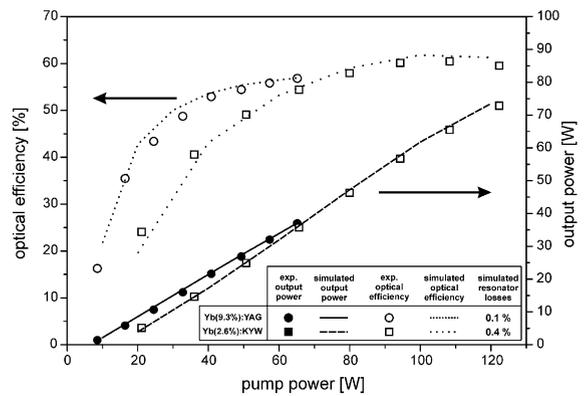
Fig. 4. Input–output curves and optical efficiencies of Yb:YAG and Yb:KYW; the full and dashed lines are calculated curves and the full and open symbols are experimental data.
