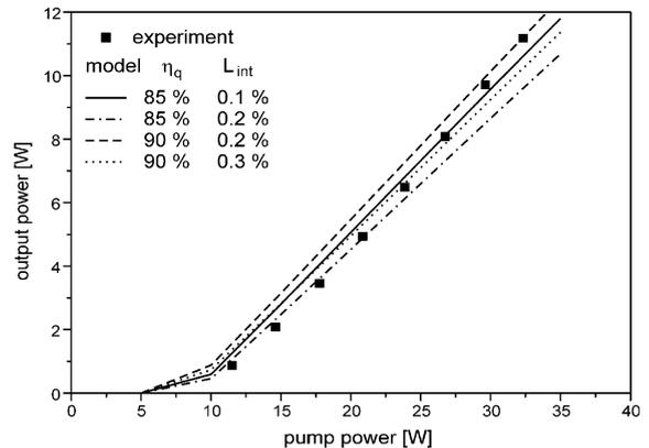
Fig. 5. Input–output curve of Yb:Lu<sub>2</sub>O<sub>3</sub> and corresponding simulation calculations; the best fit is obtained with 85–90% quantum efficiency.
