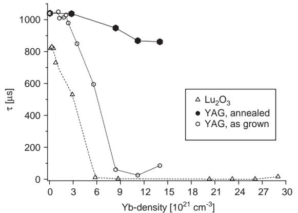
Fig. 2. Fluorescence lifetime of Yb:YAG and Yb:Lu<sub>2</sub>O<sub>3</sub> versus Yb concentration.
