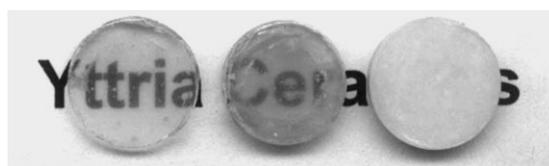
Fig. 9. Photograph of  $Y_2O_3$  ceramics (a) striking at 0 °C (b) striking at 50 °C and (c)  $SO_4^{2-}$  undoped.
